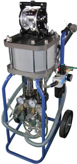
TP4SS Pump is a high pressure, high volume airless pump with a fixed ratio of 1:1 for automatic mixing systems. It is used in the construction and mining industry for the injection of polyurethane and is especially suited for high volume water control, void filling and deep injection applications. The TP4SS Pump incorporates a flush pump and flush pump feed line to the mixing head allowing for fast and efficient cleaning of the mixing head between breaks in the injection sequence.
